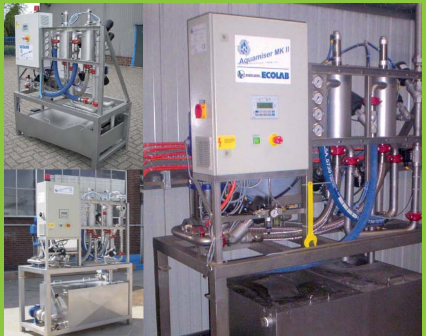
The Aquamiser filters water to achieve savings through reuse of "cleaned" water. The system removes lint, sand and other particles down to 25µm.
